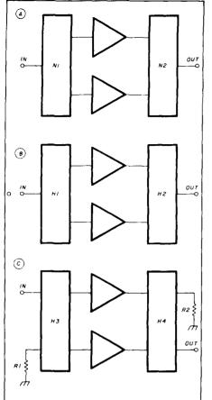
fig. 6. Various schemes for high power with combining networks. (A) in phase technique. N1 and N2 are reactive splitters; (B) H1 and H2 are 0 or 180-degree hybrid transformers. (C) H3 and H4 are 90-degree hybrid transformers. R1/R2 are 50-ohm loads. Resistor power rating depends on input or output power levels.
